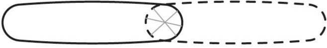
Fig. 4. Degenerate case where there is an infinity of witness pairs (some pairs are depicted in gray).
