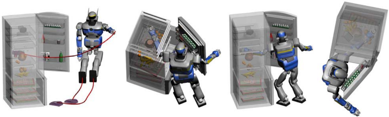
Fig. 18. Pick-can-from-fridge scenario. From left to right: illustration of the target, posture obtained without collision avoidance constraints, successful free-collision posture found (side and up views).
